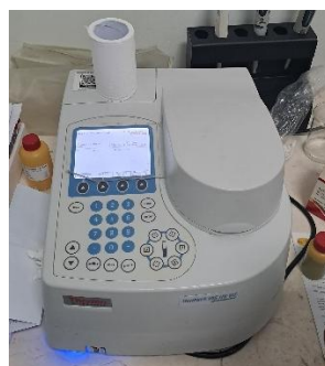
Spektrofotometri Thermo Scientific Genesys 10S UV-VIS
