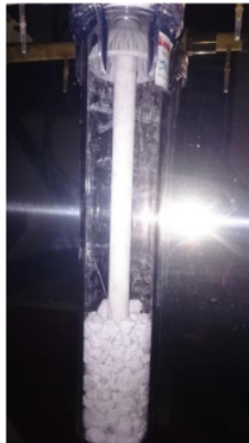
Figure 2. The filter housing contains lime granules on a portable fume hood.
