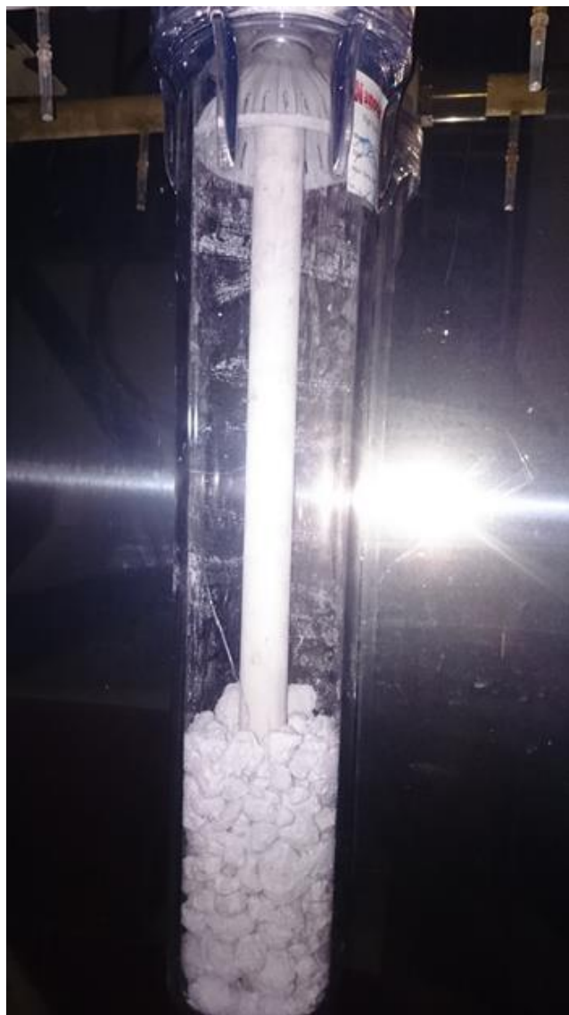
Gambar 4.3. Housing filter berisi granul kapur pada fume hood portabel
