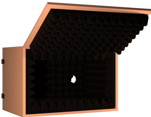
Gambar 4. Desain 3D Silencer Box tampak samping
