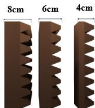
Gambar 8. Desain Variasi Ketebalan Media Egg Tray
