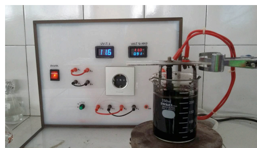
Figure 3. Coal Desulphurization by Electrolysis Method
