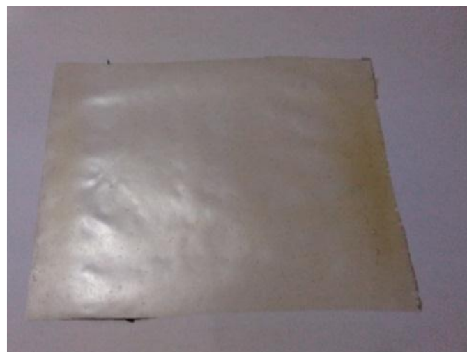
Figure 3 Bioplastics produced a sheet of thin and transparent
